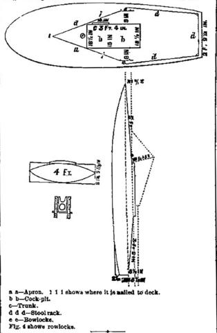
**Figure 5.** The first printed description of a Barnegat Bay Sneakbox appeared in Forest and Stream on April 3, 1874, in a short letter from Robert B. White, including a rough dimensional drawing. (Courtesy New Jersey Department of Environmental Protection, Double Trouble Village State Historic Site archives, 1874)
